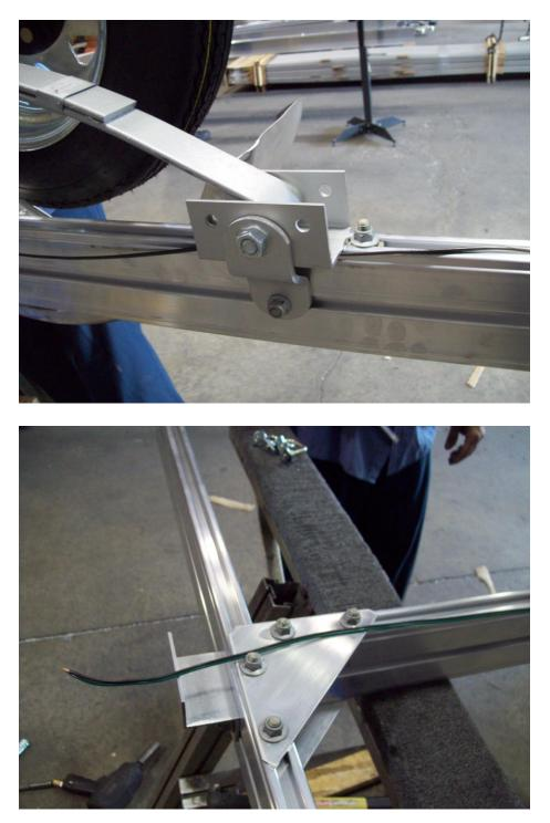
Route the wires through the channel and around the leaf springs to the back of the trailer. Make sure to leave enough harness for the rear tail light then cut off the excess wire. Be sure to keep left over harness, this will be used later.
