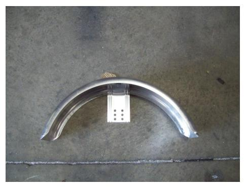
Locate the fender with mounting bracket.
