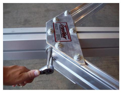
Slide tongue into position on the frame and tighten nuts.
