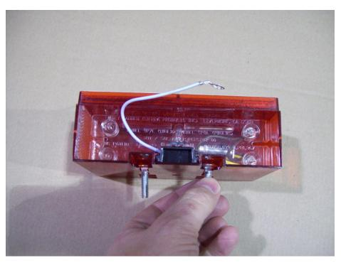
Install carriage bolts into the back of the tail lights as shown.
