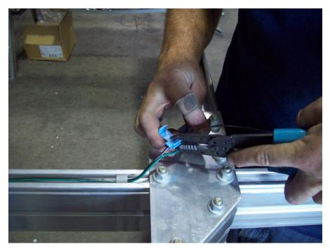
Use pliers to push the metal spade down until it is flush with the plastic. This is what makes the electrical connection between the two wires. Close the plastic cover of the connector over the spade until it snaps into position.
