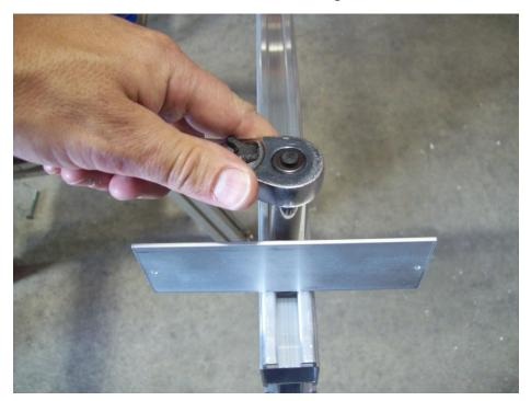
Slide side marker brackets into each side of the front cross member. Position them about 1" in from each end of the cross member and then tighten.
