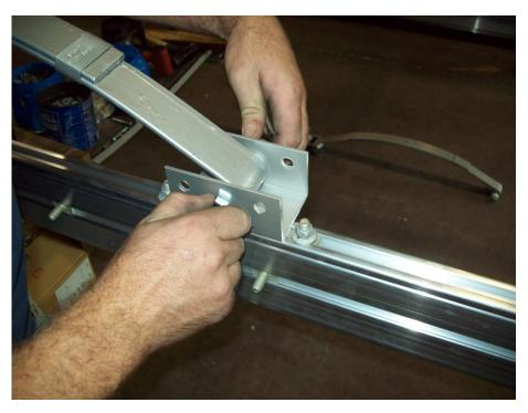
Remove the bolt from the front spring eye and install the spring into the spring hanger in the center hole with the nut towards the inside of the trailer. Do not tighten yet.
