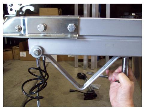
Slide bracket into the bottom channel of the tongue section. Position bracket as shown and tighten nuts.
