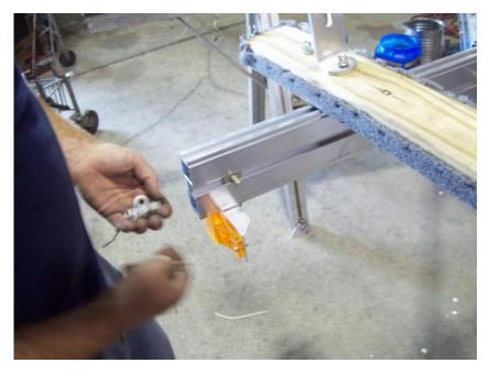
Slide one T-bolt on each side of the front and rear crossbar to mount the angle brackets.
