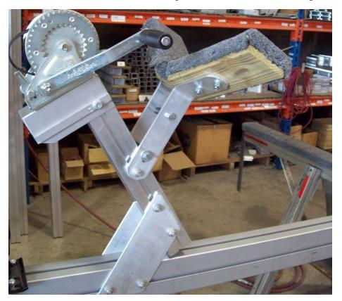
Now install winch post onto angle braces as shown. Once final placement has been determined tighten nuts on angle braces.
