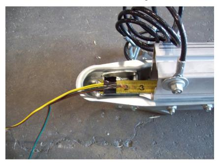
Attach both wires of the harness to the end of the tape measure with either tape or a tie. Retract the tape measure until it comes out the back of the tongue with both wires attached.
