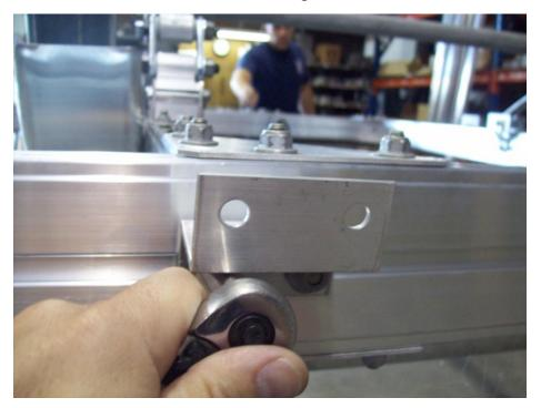
Slide the brackets into the rear cross member. Position as shown.
