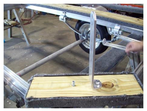
Locate the transom bunk and install slotted angle bracket to it as shown.
