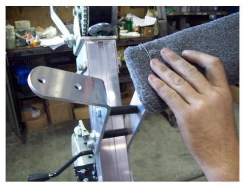
Install the bunk boards to the angle brackets of the winch post.
