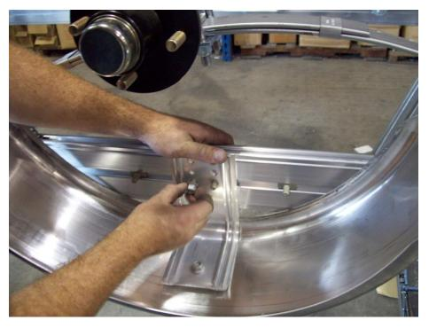
Position the four T-bolts on the side rail under the axle as shown. Install the fender bracket over the two inner T-bolts. Then position and tighten nuts.
