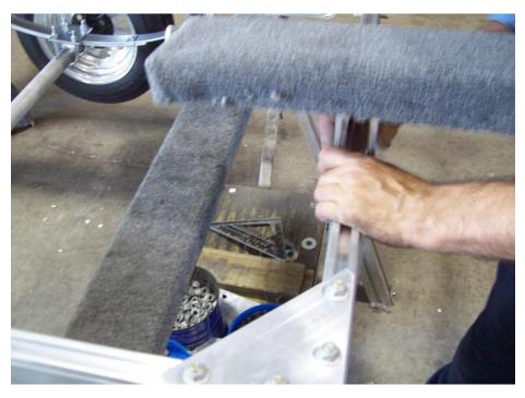
Install both transom bunks on the rear crossbar and center them. Install slotted angle bracket and tighten nuts.
