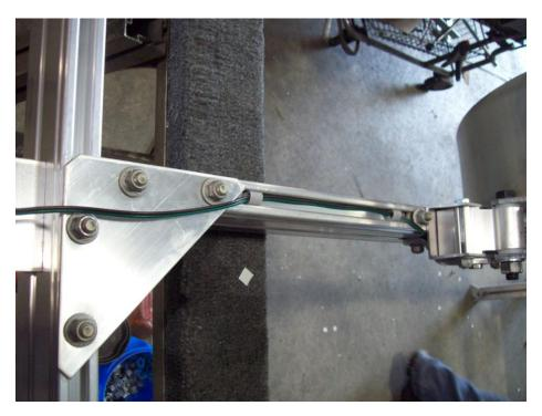
After wire is run through the channels go back and add adhesive clips to take up the slack on the harness as shown.
