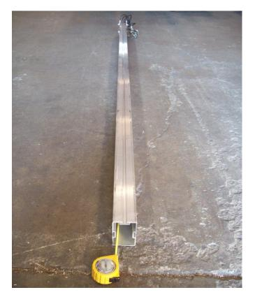
Extend a tape measure inside the tongue from the rear of the trailer until it protrudes at the front of the trailer under the coupler.
