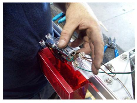
Install the tail lights to each bracket. Make sure to tighten nuts but don't over tighten them. Loosen the wire retaining screws and install the color matching wires from the wire harness onto the corresponding retaining screws.
