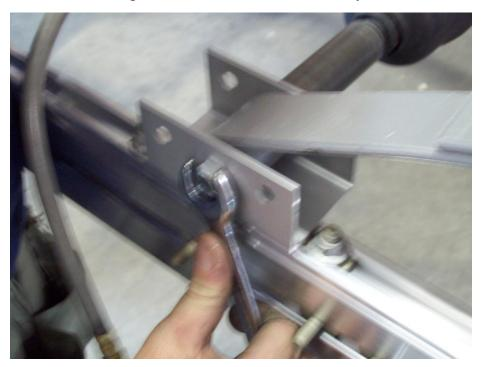
Now go back and first tighten the front spring mounting nuts that were left loose previously.
