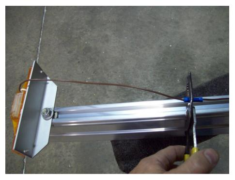
Take the brown wire from the running light and insert it into the butt connector and crimp it on.
