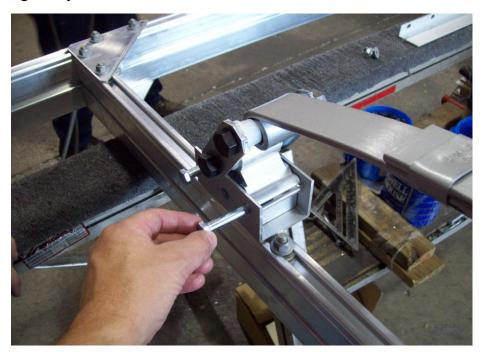
Remove the two bolts from the shackle holder at the rear of the spring and install the shackle holder into the rear spring hanger with the nuts toward the inside of the trailer then tighten the nuts. Do not tighten the shackle nuts yet.
