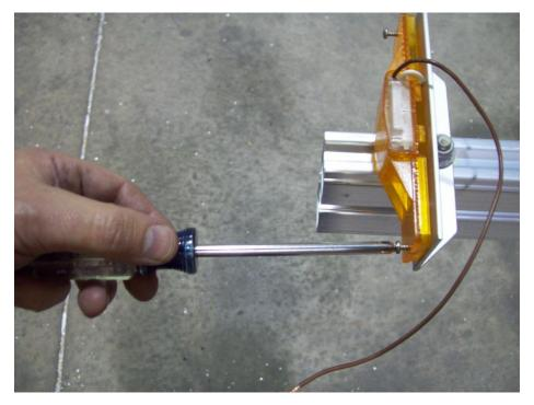
Install the running lights into the pre-drilled holes in the running light bracket using a Philips screwdriver. Be sure the screw is through the ring terminal on the back side of the lights. This will supply a ground to the lights. <u>DO NOT OVER TIGHTEN</u>
