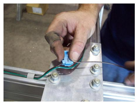
Insert brown wire that has been cut into the hole in the connector closest to the hinge. This hole does not pass all the way through. The wire should go in about  $\frac{1}{2}$ ". Pass the other wire through the remaining open slot in the connector.
