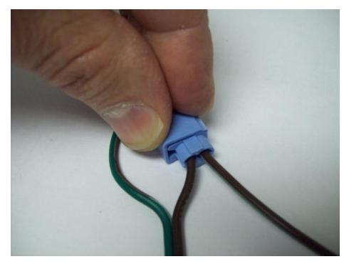
Close the hinge cover on the connecter, this finishes the process. This illustration is used in the next step for wiring the side marker lights.
