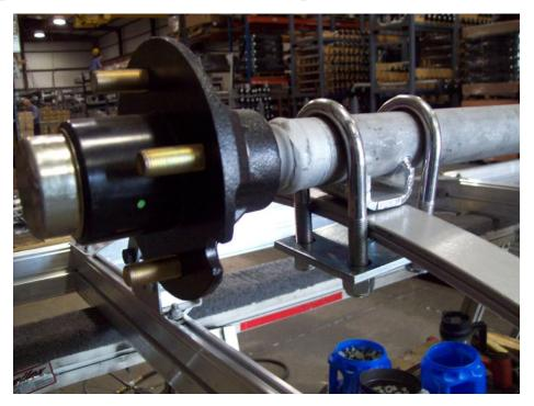
Locate the U-bolts and tie plates and install them as shown.
