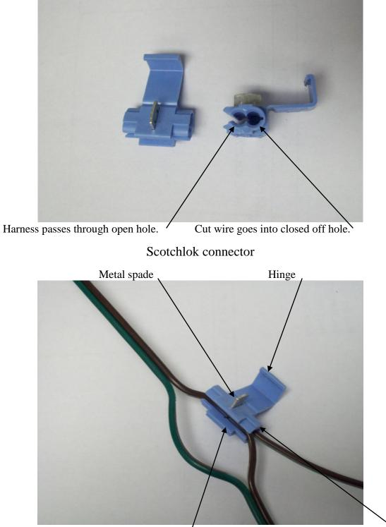
Harness shown passing through open slot. Cut wire from side light in closed section.
