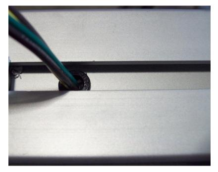
Once harness is through the grommet it can be snapped in to position.
