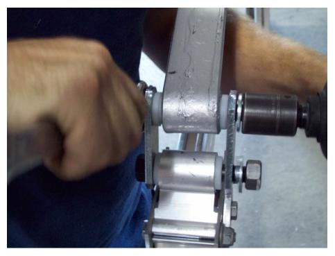
Then tighten the rear shackle nuts. Do not over tighten as this will not allow the suspension to move properly.
