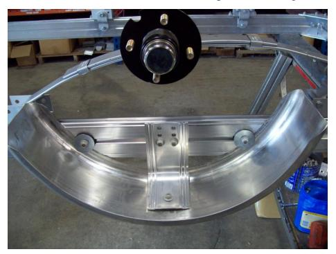
Install the washers over the outer two T-bolts. First two rubber washer, two steel washer and nuts. Slide T-bolts and washer over the inside edge of the fender then tighten nuts.
