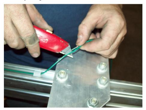
Separate the green and brown wire as shown on the front cross member. This is to splice the side marker light into the harness. Repeat the process for the other side.
