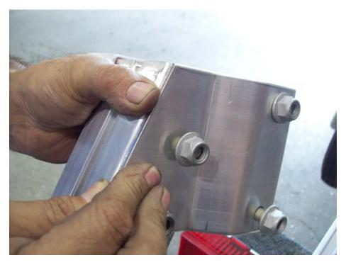
Install both top offset attaching plates to rear gusset and position as shown.
