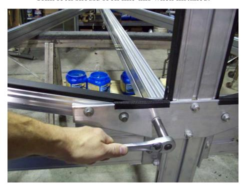
At this point tighten all nuts on arm assemblies.
