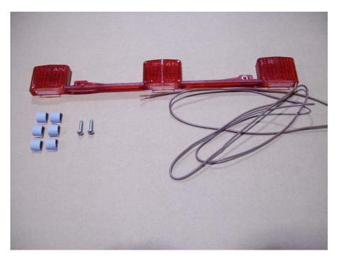
Locate the three light bar, adhesive clips, and two large Philips screws.
