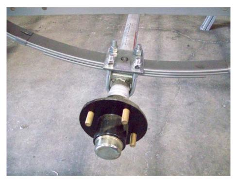
Position the axle and tighten the nuts evenly on the U-bolts.
