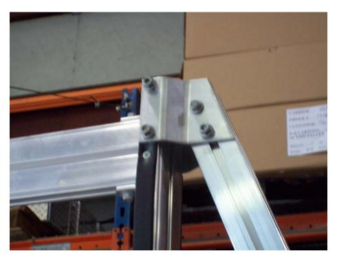
Insert T-bolts from the top offset attaching plates into the vertical post.
