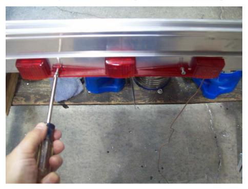
Install the three light bar on the rear cross member in the center where the holes are drilled.
