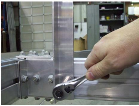
Slide the outer T-bolts in the cross member over to the corner angle bracket. Install support angle bracket over top of T-bolt. Support angle bracket should be flush with corner angle bracket. Tighten nut.
