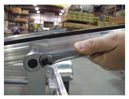
Tighten nut on arm assembly. Repeat this process for all four corners.
