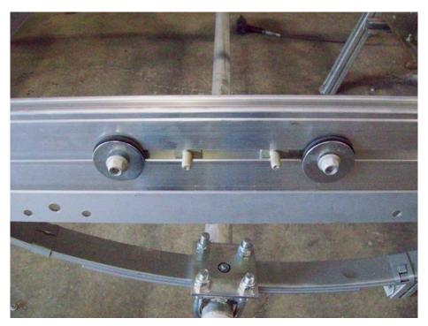
On the side rail of the trailer, locate the T-bolts and washers to mount the fenders.
