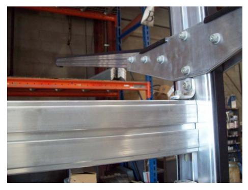
Loosen the lower angle brackets and slide out of the way. Insert top T-bolts into the upper angle brackets as shown and install nuts. Reattach lower angle brackets to underside of the bar. Install nuts and tighten.
