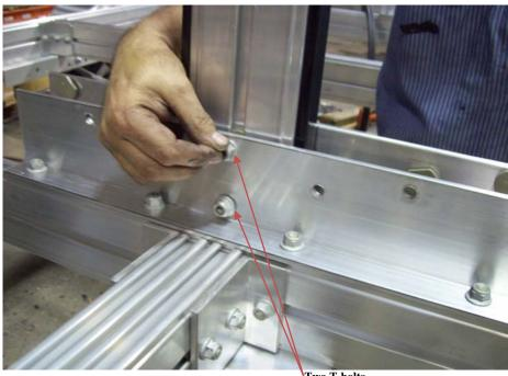
Install the two T-bolts on the front side of the post into the bracket on the cross member as shown. Install nuts, and then tighten the front and back. Repeat the process for the rear post.
