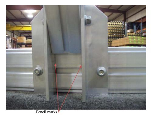
Loosen angles and slide down over T-bolts. Attaching angles should line up with pencil marks on rear cross member. Reinstall nuts on T-bolts.
