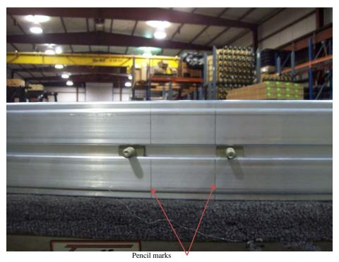
Remove nuts on the front side of the rear cross member. Position T-bolts on each side of the pencil marks.
