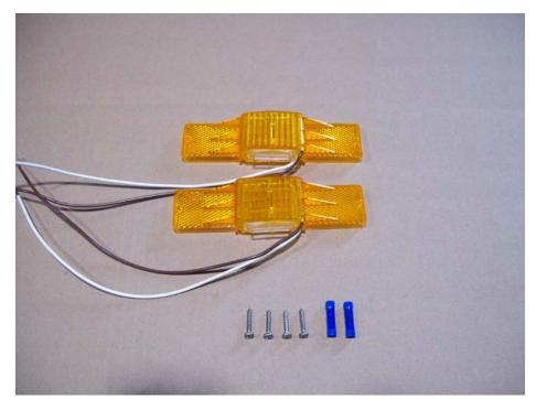
Locate two amber running lights, four small Philips screws, and two butt connectors.
