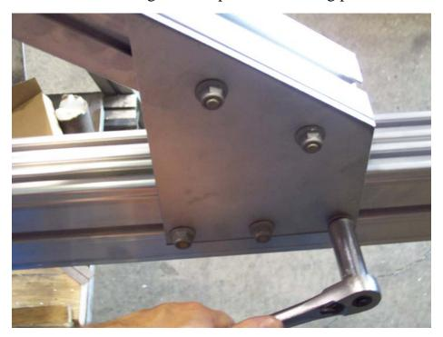
Install the right side bottom attaching plate into the three T-bolts on the tongue section. Now go back and tighten all the nuts on the top and bottom plates.
