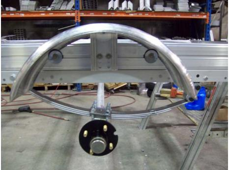
Install the fender bracket over the two center T-bolts. Slide the T-bolts with washers out against the edge of the fender as shown. Center the fender over the axle and tighten all nuts.
