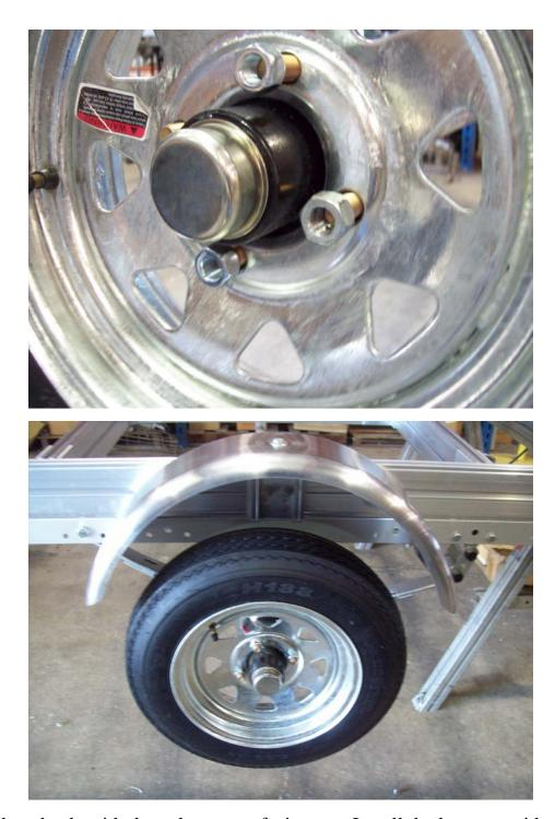
Install the wheels with the valve stems facing out. Install the lug nuts with the tapered side facing the wheel then tighten nuts.
