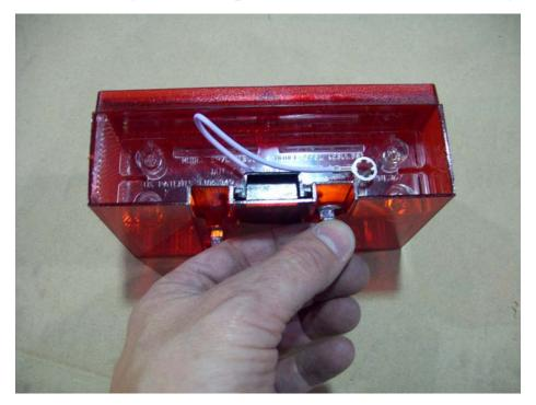
The light with the yellow wires is for the left (driver's side) of the trailer. Slide the carriage bolts into the slots in the back of the tail lights.
