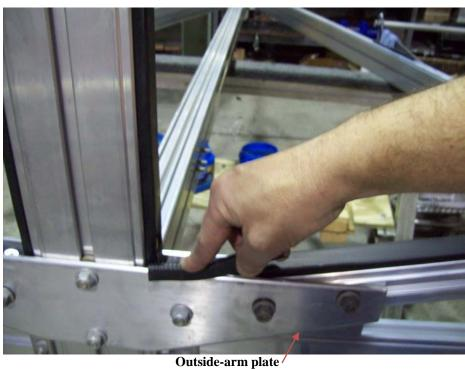
Push the trim lock down on the outside-arm plate as shown. The trim lock will not be used on the front side of the arms. Repeat this process for all of the outside plates.
