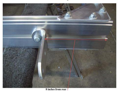
Install tail light brackets on T-bolts that are already on the side rail. Position tail lights 8 inches from the rear cross member as shown.
