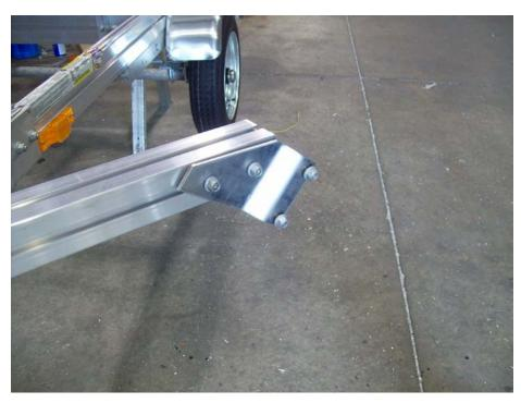
Install only the left side top plate. Position plate and tighten nuts.
