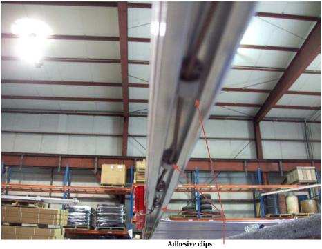
Take the wire from the three light bar and run it across to the right side tail light. Tuck the brown wire up into the underside of the cross member and install adhesive clips as shown.
