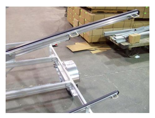
Repeat the process of installing the web strap clips for the top cross bars. Final adjustments to clips will be determined when boats are loaded on trailer.
