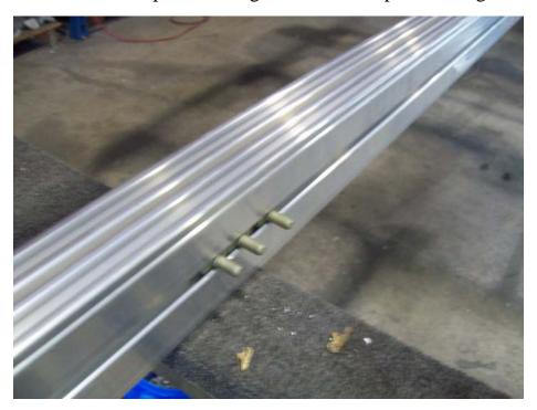
Locate the three T-bolts on the tongue section. Remove nuts and slide them towards the front.
