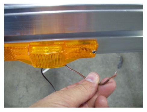
Locate the two drilled holes at the front of the side rail and install the light. Then strip away about a 1/4" of casing off the brown wire from the light.
