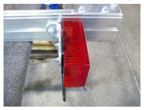
Install the left tail light with the license plate holder between the light and the bracket. Repeat the process for the other side then tighten the nuts on tail lights.
