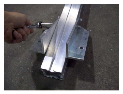
Install both of the bottom attaching angles to the gusset. Slide both angle plates about 2-3" up on the gusset and snug the nuts.
