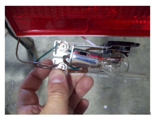
Remove the tail light assembly from the housing. Loosen the wire retaining screws and install the color matching wires from the wire harness onto the corresponding retaining screws. Reinstall into the housing. Repeat process for the other side.
