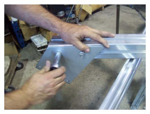
Install the left bottom plate to the gusset. Position plate and tighten nuts.
