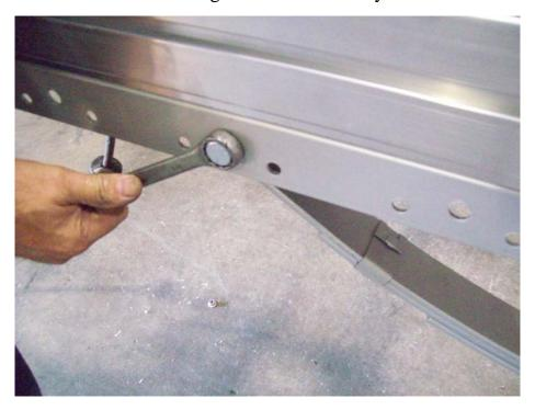
Once the axle is installed, go back and tighten the nuts on the leaf springs.
