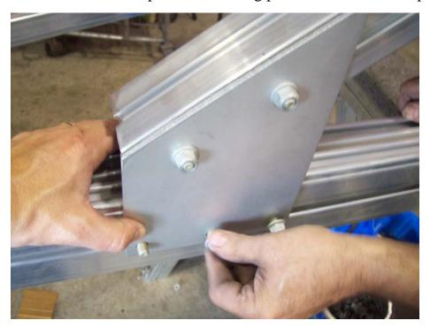
Install the bottom attaching plate onto the three T-bolts on the tongue section. Reinstall nuts but don't tighten yet.
