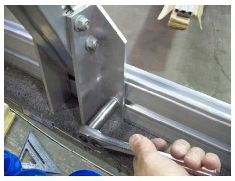
Now go back and tighten nuts on both top and bottom plates.
