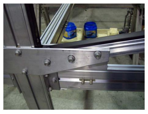
Insert the arm into the T-bolts on the brackets. T-bolts will need positioned to accommodate the arm as it is sliding in toward the post.
