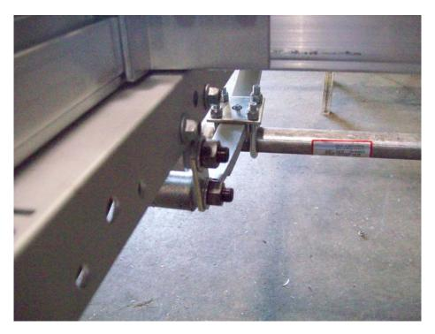
Do not over tighten the shackle nuts as this will not allow the suspension to move properly.
