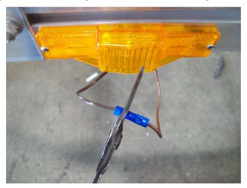
Pull down the brown wire of the main harness from the underside of the frame and strip ¼" of casing off this wire. Crimp butt connector to both wires.
