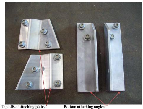
Locate two top offset attaching plates and two bottom attaching angles for the rear gusset.
