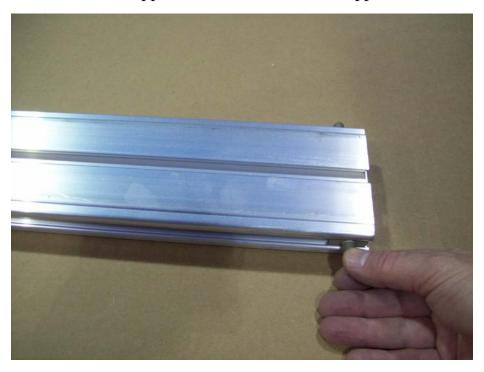
Remove the T-bolts from the angle brackets located halfway up on the back side of the vertical support. Install one T-bolt in each corner of the lower horizontal support.
