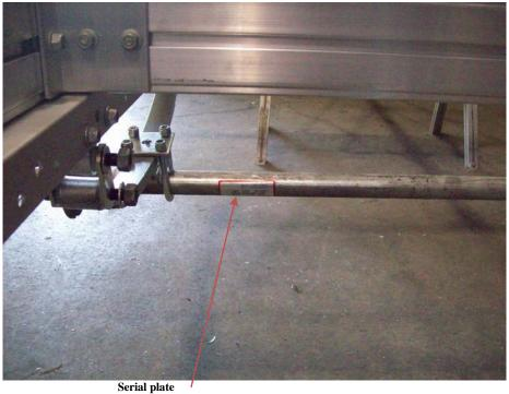
Install the axle making sure the locating studs on the springs are in the holes on the axle's spring seat. Face the axle's serial plate toward the rear of the trailer to protect it from debris. Install the axle using the U-bolts, plates and nuts.
