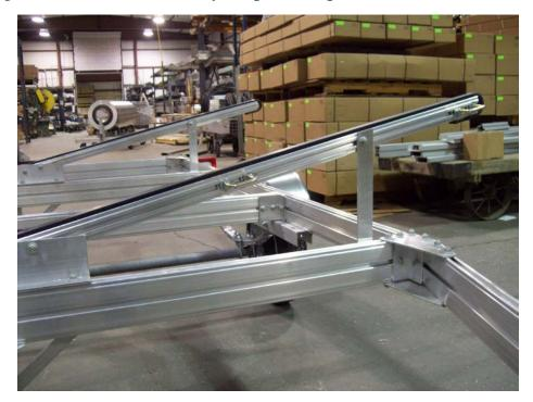
Install web strap clips at the end of each cross bar as shown and tighten.
