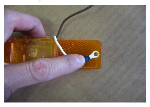
Align the ring terminals with the screw hole nearest the wire on the back of the running light. Make sure the wire is routed through the gap on the back of the light so it does not become pinched, when the light is installed.
