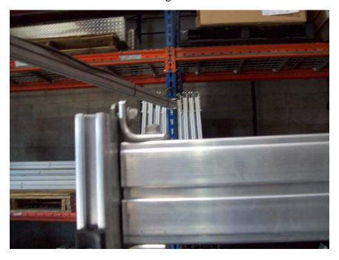
Install the upper horizontal bar into the top of each vertical post.
