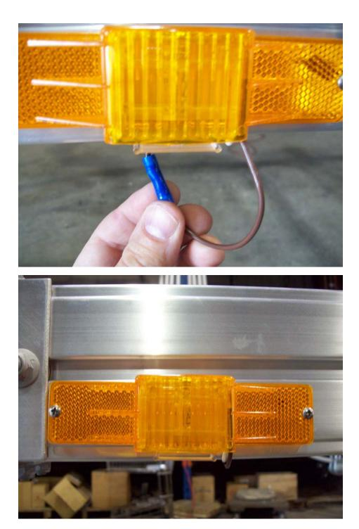
Insert the wire and butt connector into the hole on the underside of the rail. The wire should not be visible once inserted into the frame.
