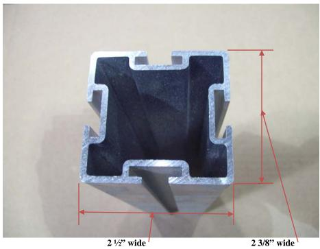
The front and rear gusset bars are not a perfect square. One side is  $2\frac{1}{2}$ " wide the other is  $2\frac{3}{8}$ " wide. The attaching plates will be mounted to the side that is  $2\frac{3}{8}$ " wide.
