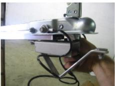
Slide the running light bracket into the bottom slot in the front tongue section.
