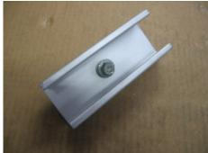
Locate the running light bracket with bolt and nut.
