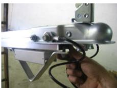
Slide the front of the skid into the bottom slot in the front tongue section.
