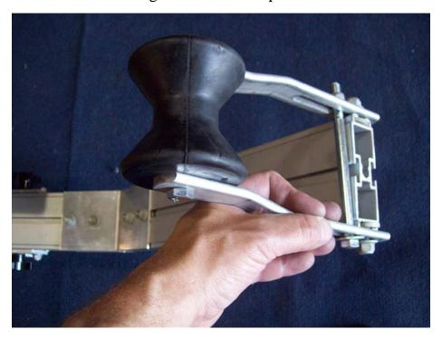
Install bow stop on front tongue section as shown.
