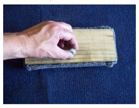
Locate the 10" padded cradle and remove the lock washer and nut from the backside.
