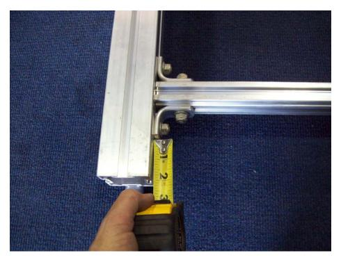
Position the axle spacer 2" away from the end of the axle.
