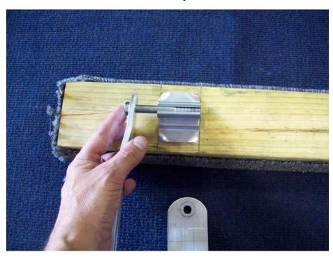
Locate the 48" padded cradles and offset brackets. Install the 3 1/4" bolts through the slotted brackets and pivot as shown. Repeat this process for the other padded cradle.
