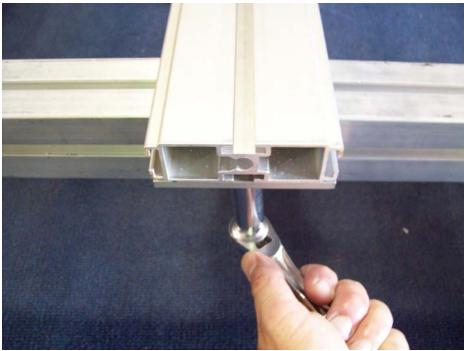
Insert the tongue section through the T-bolts on the angle brackets of front axle. Tongue section should slide through all the way to the rear axle angle brackets. Rear tongue section should be even with the rear angle bracket as shown. Tighten all nuts at this point.
