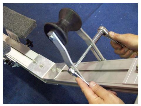
Position bow stop and tighten nuts. Finial adjustments will be made when boat is on dolly.
