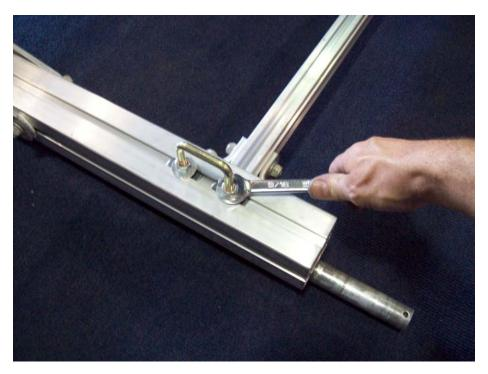
Install a web strap on each side of the front axle as shown. Tighten nuts at this point.
