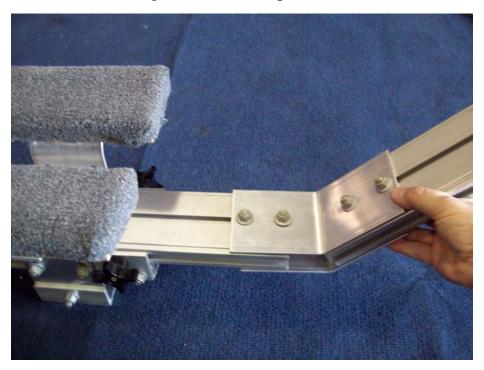
Install front tongue section into tongue as shown.
