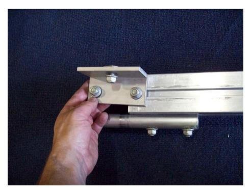
Install the angle bracket on the axle assembly as shown and slide towards the center.
