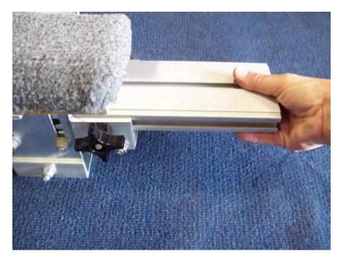
Loosen the knobs on both sides of the tongue section. Slide the tongue section out enough to attach the front tongue section with plates.
