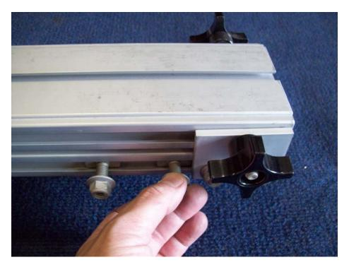
Remove the nuts from both sides of the lower tongue section. Make sure the four prong knobs are on the upper tongue section as shown.
