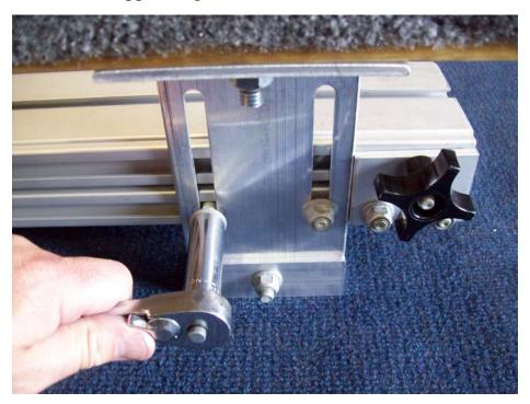
Install cradle assembly over bolts on tongue section. Reinstall nuts and tighten.
