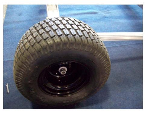
Install the wheels with the valve stems facing out.
