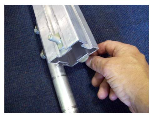
Install two T-bolts on both sides of the axle assembly and repeat for other side.
