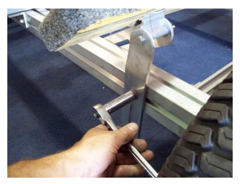
Go back and adjust and tighten the nuts for the cradle brackets. Final position will be made with the boat on the dolly.
