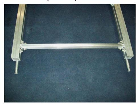
Install the other axle and position as shown. Repeat the process for the other side.
