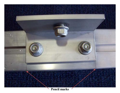
Align the angle bracket between the pencil marks on the axle assembly.
