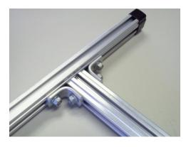
(Pencil marks.) Install 3 cross bars to the T-bolts in the wide sides of the uprights. Align the center of the cross bars with the pencil marks on the uprights.
