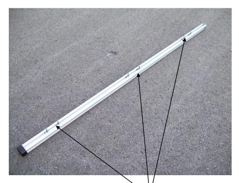
Lay out the four 66 inch uprights and install 6 T-bolts in the wide side and 4 T-bolts in the narrow side of each. (Pencil marks.)
