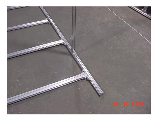
Install the 4 cross bars that hold the two rack sections together on the "narrow" side of the uprights at the pencil marks.
