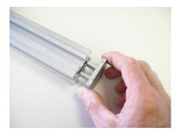
Install a vinyl cap and aluminum foot on each end.
