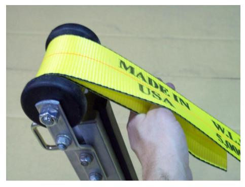
At this point, pull inner strap to raise it up off the axle assembly.
