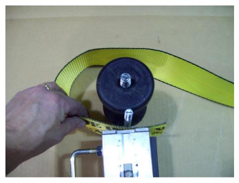
Start with the left side of the upright assembly now. Take the strap and loop it over the top of the roll, then run it down under the bottom bolt.
