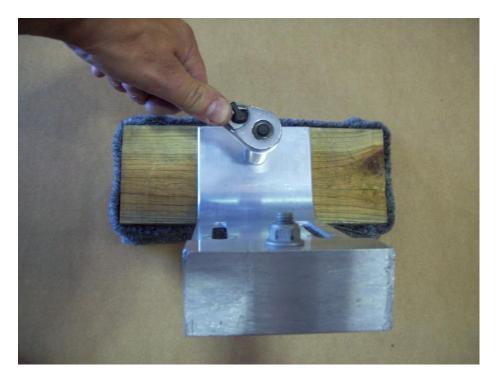
Install skid bracket on the bottom of the padded cradle as shown. Reinstall lock washer and nut then tighten.
