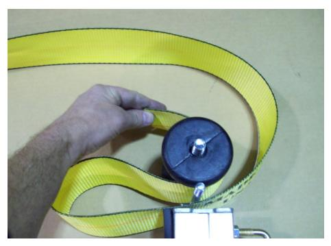
Guide strap around the backside of the roll, and then bring it over the top of the roll. Pull about a foot of the strap through at this point.
