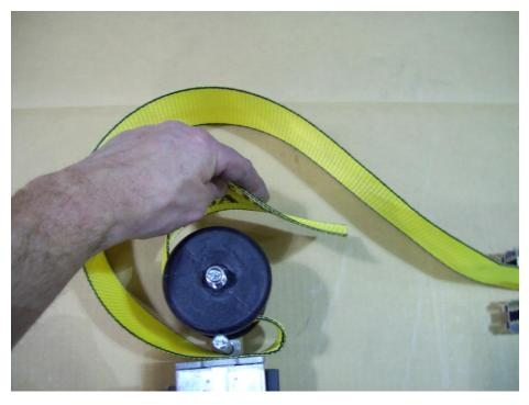
Guide strap around the backside of the roll, and then bring it over the top of the roll. Pull about a foot of the strap through at this point.
