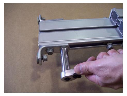
Align angle bracket flush with the end of the tongue section as shown. Tighten nuts on both sides.
