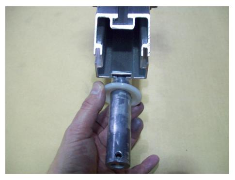
Install one nylon retainer washer on the axle with the grooved side facing out.
