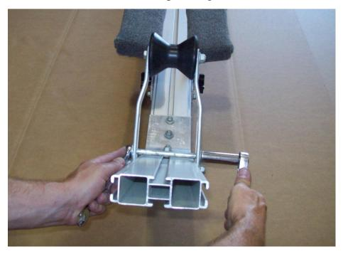
Tighten bolt and nut against the tongue section as shown. Final adjustments will be made when the boat is on the dolly.
