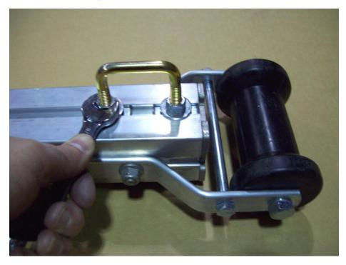
Once web strap clip is in position tighten nuts. Repeat this process for the other side.
