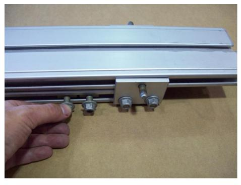
Remove the nuts from both sides of the lower tongue section.
