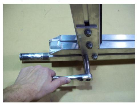
Make sure the bottom of the upright assembly is flush with the axle assembly. Once in position tighten nuts and repeat the process for the other side. These nuts will need to be torqued to 35-40 ft. lbs. Final position will be determined with the boat on the dolly.
