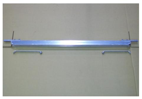
Axle assembly and diagonal struts.
