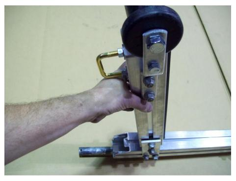
Insert upright assembly into T-bolts on the brackets as shown. The rubber pads on the upright assembly should be facing inward.
