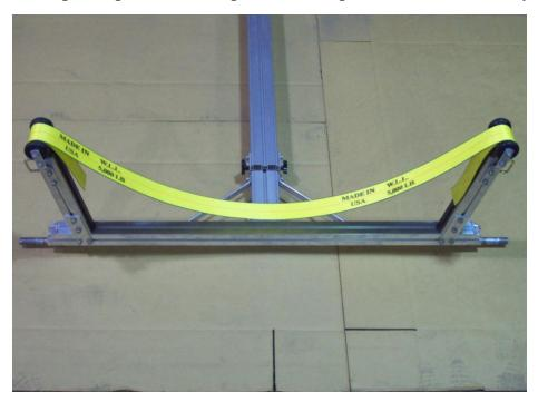
The strap should not be touching the axle assembly when finished.
