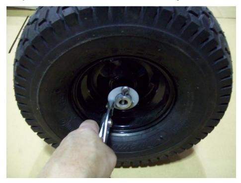
Install the wheel with valve stem facing out. Install the nylon washer on the axle with the grooved side facing in. Insert cotter pin and bend the ends so it doesn't come out. Repeat this process for the other side.
