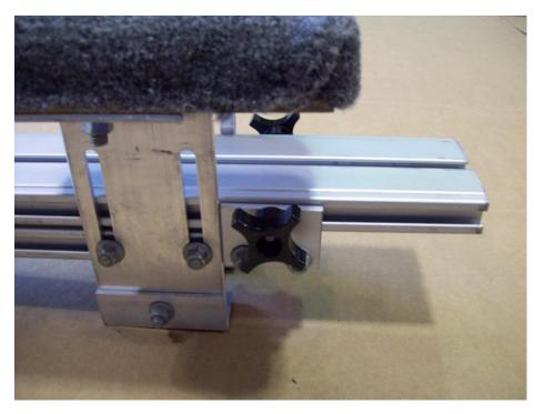
Install 2 four prong knobs on the upper tongue. Leave knobs loose for now until finished.
