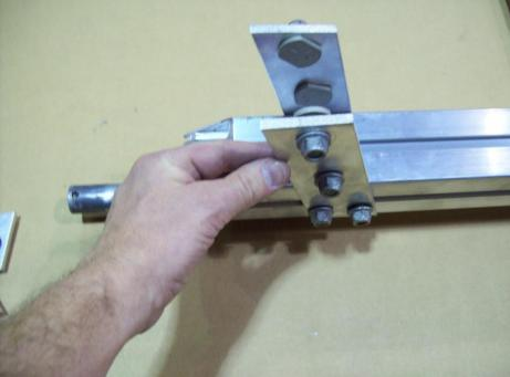
Insert the upright attaching brackets into the axle assembly. Position the bracket about 2" inward on the axle assembly. Make sure the brackets are tilting outward once in position. Do not tighten nuts at this point.
