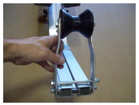
Install bow stop on front tongue section as shown.
