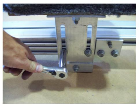
Install cradle assembly over the bolts on tongue section. Reinstall nuts and tighten.
