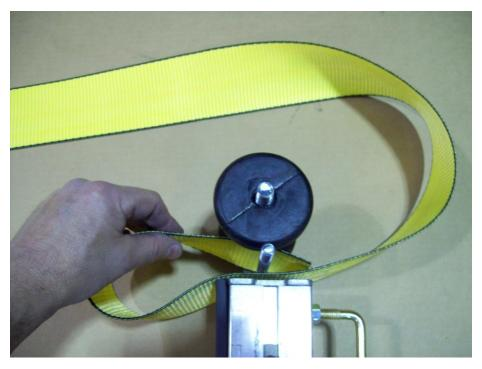
Once under the bottom bolt, pull strap through and loop it back over the top of the bottom bolt as shown.
