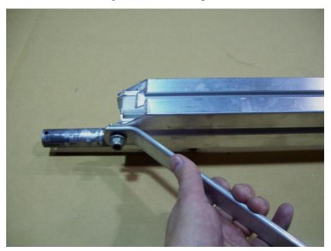
Slide strut onto axle as shown.
