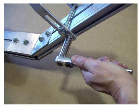
Position bow stop and tighten nuts.
