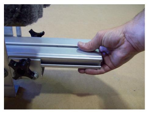
Slide the upper tongue section out enough to attach the front tongue section with plates.
