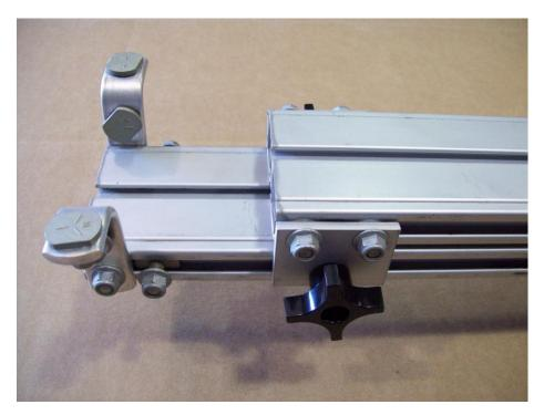
Install the other 2 four prong knobs on the lower tongue section. Leave knobs loose for now until finished.
