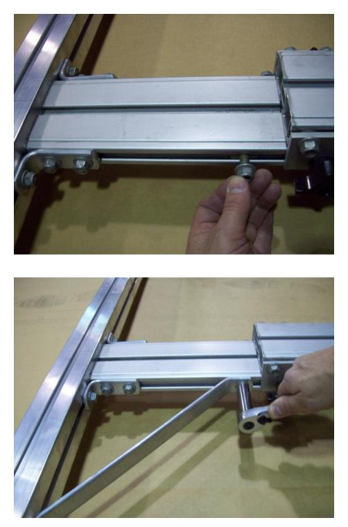
Remove nut from T-bolt on tongue section and install strut. Reinstall nut, position strut and tighten nuts. Repeat the process for the other side.
