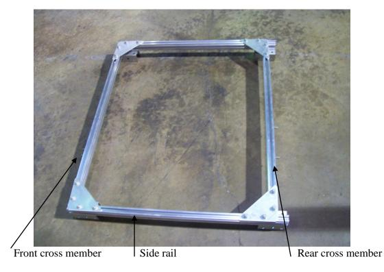
Next layout the front and rear cross member and slide the side rails through them to make a square frame as shown.
