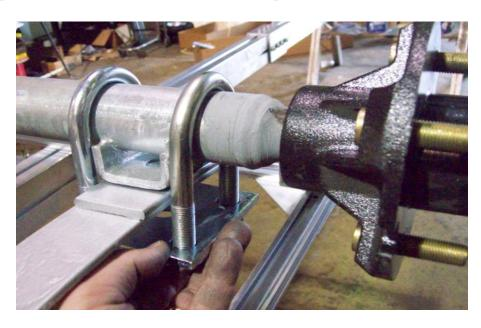
Locate the U-bolts and tie plates and install them as shown.
