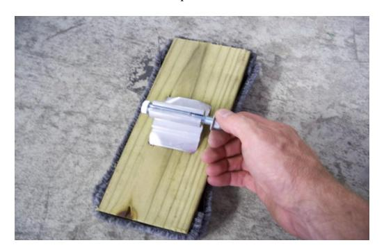
Remove the bolt from the pivot plate.
