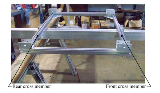
Frame attached to the tongue section shown up side down.
