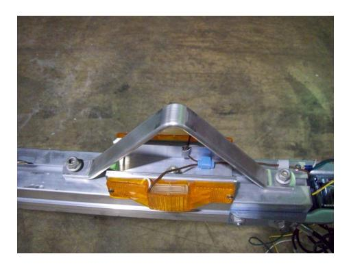
Install the skid on the front tongue section now. Tighten the nuts for the skid in the location as shown. Turn the trailer right side up at this point.
