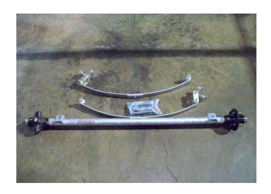
Axle assembly, springs and U bolt hardware.
