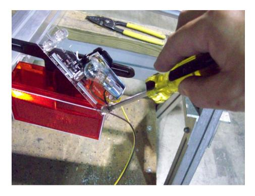
Loosen the wire retaining screws and install the color matching wires from the wire harness onto the corresponding retaining screws.
