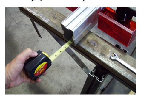
Extend a tape measure inside the tongue from the rear of the trailer until it protrudes at the front of the trailer under the coupler.
