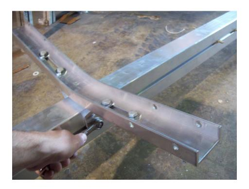
Using the rearward most bolts of the three that were moved toward the coupler during tongue assembly, attach the front cradle holder assembly at the pencil marks located 36" from the front of the tongue. Final location of the front cradle holder will be determined when the boat is fitted to the trailer.
