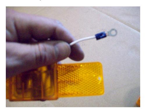
Install the ring terminals by crimping the terminal onto the bare wire.
