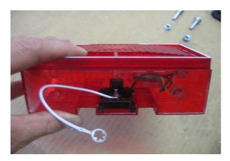
The light with the yellow wires is for the left (driver's side) of the trailer.
