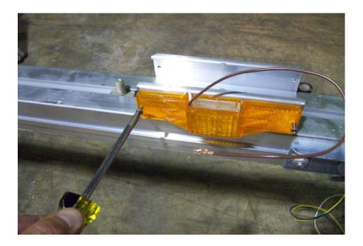
Install the running lights into the pre-drilled holes in the running light bracket using a Philips screwdriver. Be sure the screw is through the ring terminal on the back side of the lights. This will supply a ground to the lights. <u>DO NOT OVER TIGHTEN</u>
