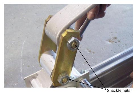
Note: The threads on the shackle link will not protrude through the shackle nut when it is properly installed. This is normal. The indentations on the flat sides of the nuts are the locking mechanism. Do not over tighten as this will not allow the suspension to move properly.
