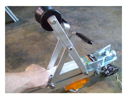
Adjust bow stand and tighten nuts. Final positioning of the bow stand will be determined by your boat.
