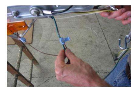
Measure 34" back from the front plug on the green/brown wire and pass the brown wire through the open slot in the second blue connector at this location. The green wire will rest just outside the connector. Insert the brown wire from the running lights into the closed side of the connector and close the spade and cover as previously described. This will make the connection from the main harness to both running lights.
