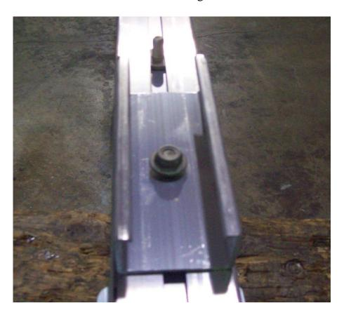
Take one T-bolt off the skid and slide it in the bottom of the tongue. Then install the bracket for the lights and position as shown.
