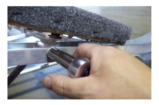
Install the padded cradle (inner position shown – this may vary depending on the width of the hull). Final angle will be determined when the trailer is fitted to the boat.
