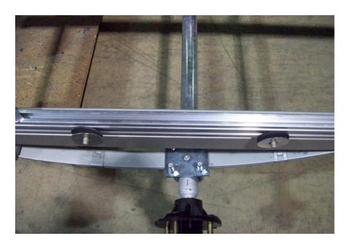
Locate (2) 1 1/8" T-bolts from the hardware bag and install them into the side rails. Slide them into position over the tire and install two rubber washers and two steel washers as shown.
