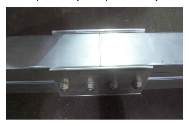
Tighten all 12 nuts making sure that the tongue sections are as tight as possible to one another. (top of tongue)
