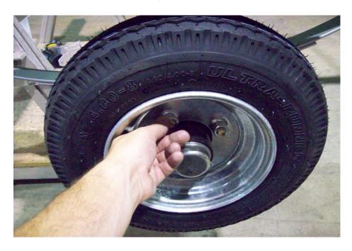
Install the wheels with the valve stems facing out. Install the lug nuts with the tapered side facing the wheel
