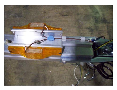
Locate the adhesive backed clamps. Install them as shown and run brown wire from the running lights through them.
