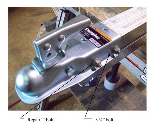
Install the repair T-bolts on the inside of the tongue to go through the front hole in the coupler. Then install nuts and make sure to tighten.
