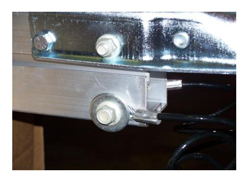
Install the repair T-bolts on the inside of the lower tongue section. Next add the cable over the bolt then a flat washer and the nut last.
