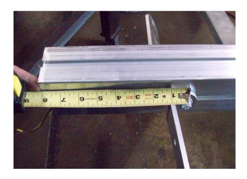
Install light bracket on both sides of the tongue section 8" from the back.
