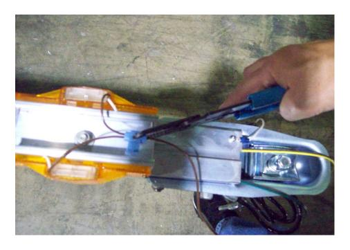
Use pliers to push the metal spade down until it is flush with the plastic. This is what makes the electrical connection between the two wires. Close the plastic cover of the connector over the spade until it snaps into position.
