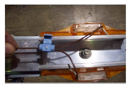
Insert brown wire that has been cut into the hole in the connector closest to the hinge. This hole does not pass all the way through. The wire should go in about ½". Pass the other wire through the remaining open slot in the connector at a point close to the running lights.
