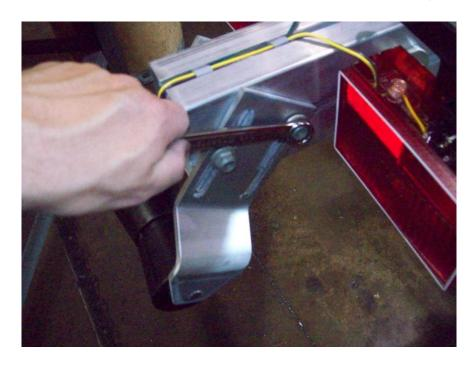
Angle the rear roll as shown and tighten all nuts. NOTICE: *The final position of this roller is such that it never touches the hull during transport – only during launch and retrieval.*
