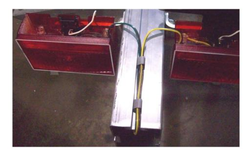
Re-install the bulb assembly into the light housing making sure to route the wires through the slot in the base of the bulb assembly. Install adhesive backed clamps in the locations shown and route the wires through them.
