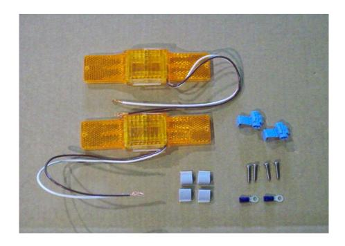
Locate the two amber running lights, four small Philips screws, adhesive backed clamps, two ring terminals, and two blue connectors.
