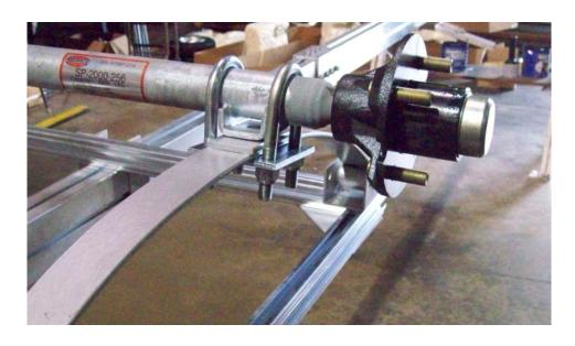
Install nuts on U-bolts. Tighten all the nuts evenly as shown in the picture.
