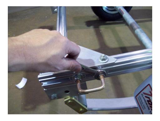
Install a web strap clip on each side rail at the back as shown. Tighten nuts.
