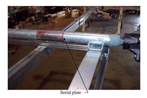
Locate the axle and install it on the springs as shown. Make sure the locating studs on the springs are in the holes on the axle's spring seat. Face the axle's serial plate toward the rear of the trailer to protect it from debris.
