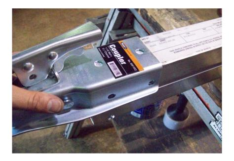
Before installing the coupler, slide 3 t-bolts on each side of the tongue. These bolts will be used later in the assembly. Now install coupler on tongue section with vin # on it, holes are pre-drilled in the tongue.
