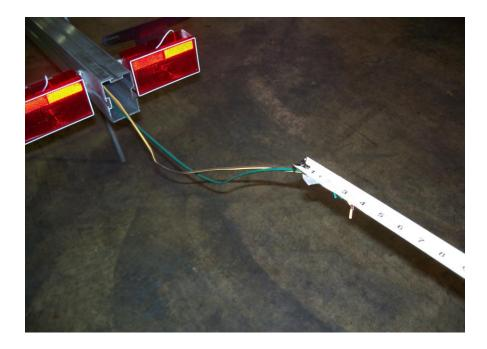
Retract the tape measure until it comes out the back of the tongue with both wires attached.
