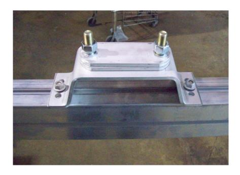
Position carrier about 18" away from the rear of the front tongue section then tighten nuts.
