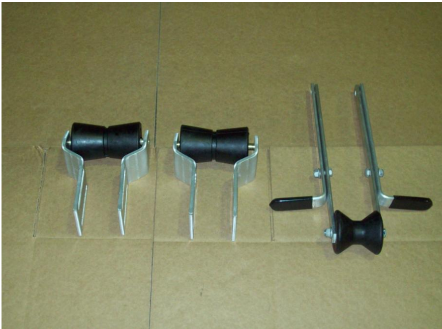
Rollers winch post and braces.
