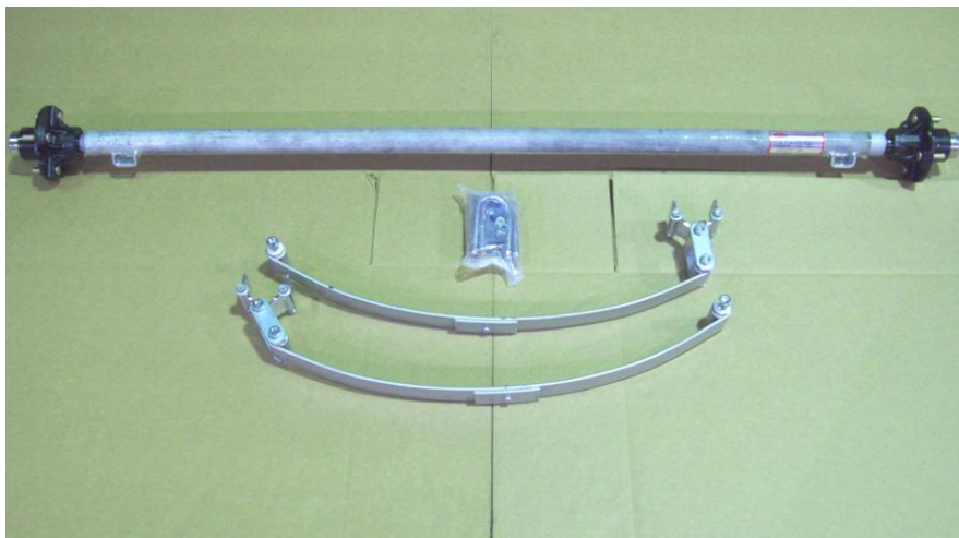
Axle assembly, springs and U bolt hardware.
