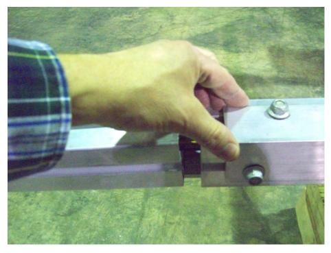
Slide the top splice plate towards the rear of the trailer as shown.
