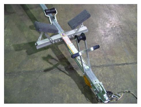
Final adjustment for the cradles will be made when boat is in position on the trailer.
