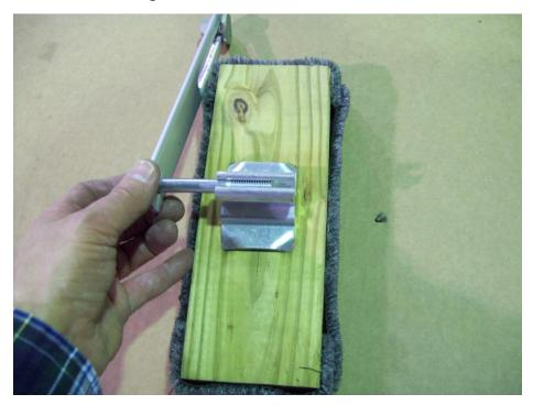
Insert bolt from the slotted bracket through the bunk pivot plate.
