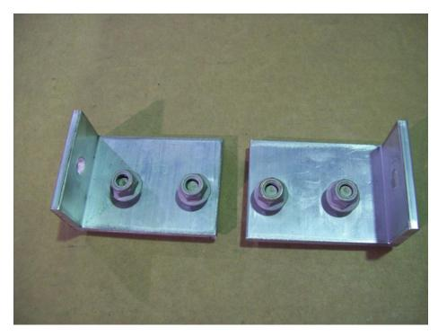
When installing the angle brackets the T-bolts will be closer to the bottom edge of the bracket.
