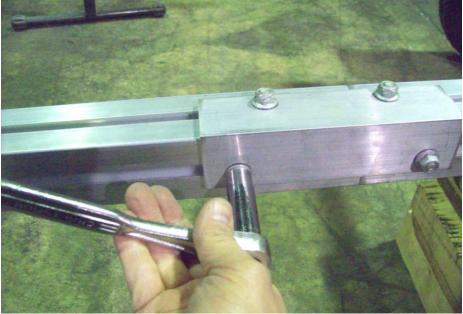
Start by loosening the nuts on the splice plate of the trailer.
