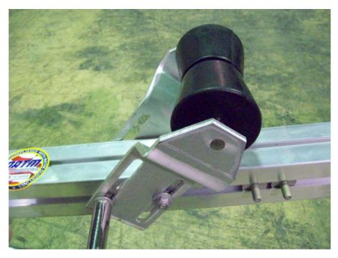
Slide two T-bolts on each side of the tongue toward the front roller. Then remove the front roller assembly. Be sure to reuse the same nuts that were installed on the roller bracket.
