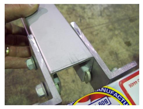
Slide the side arms into the T-bolts on the angle brackets as shown.
