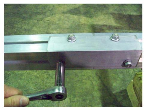
After T-bolts are in place readjust plates and tighten nuts.
