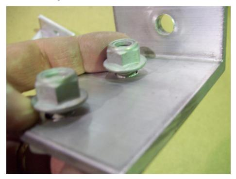
Install two T-bolts and nuts on the long side of each angle bracket.
