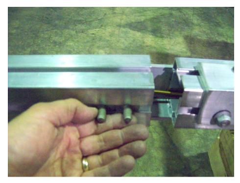
Slide two T-bolts in the front tongue sections on the left side. Then reinstall the splice plate and repeat for the other side.
