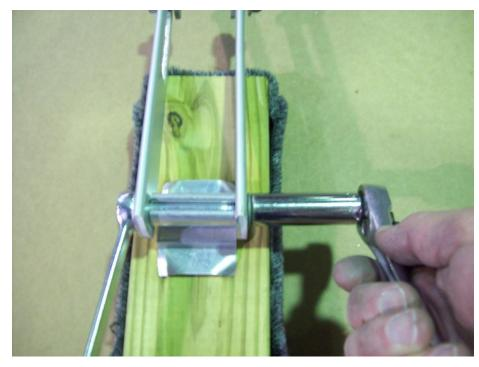
Reinstall slotted bracket and nut. Tighten so that the pad is still adjustable.
