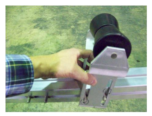
Reinstall the roller assembly on the last two T-bolts towards the rear of the tongue section. Reinstall the nuts and tighten.
