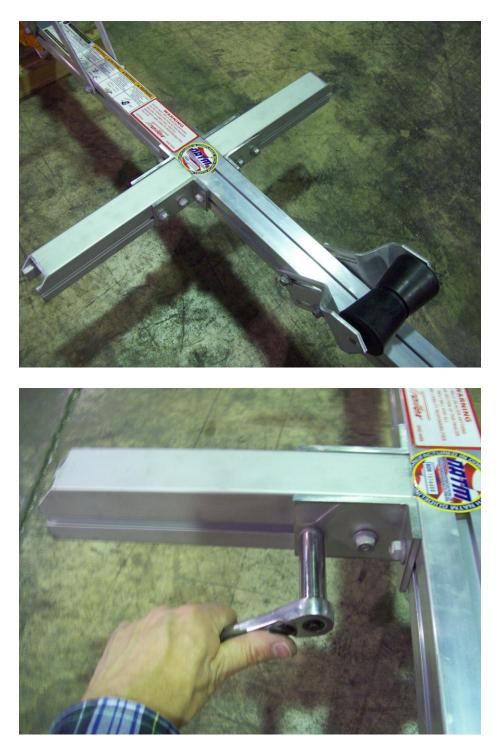
Position side arms so that they are in alignment with each other. Once in place go back and tighten all nuts.
