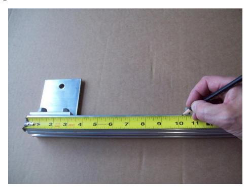
Measure in 10 ¼" from the end of the mounting bar and make a reference mark for placement.
