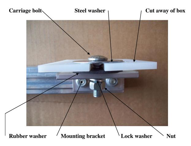
Position the box to trailer mounting brackets before drilling. Once box is position drill holes from the underside of the mount up into the box. Then install mounting hardware as shown. This completes installation of the box mount kit and box.
