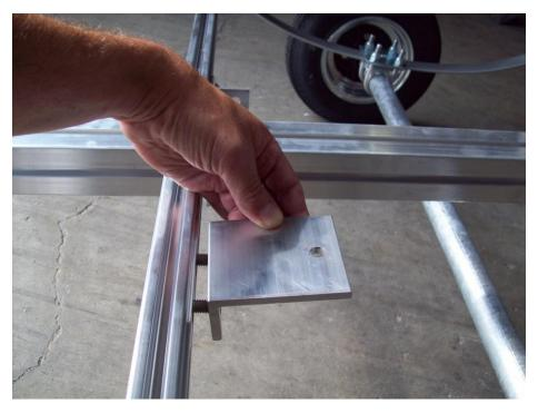
Install two repair T-bolts to each side of the front crossbar. Attach box mounting angles to each side. Install nuts but don't tighten yet.
