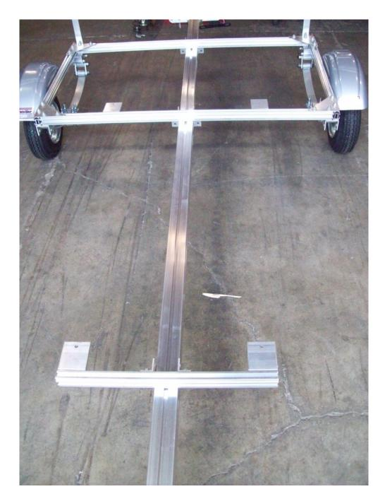
Trailer with box mount kit installed. At this point, torque all the nuts to 34 ft lbs.
