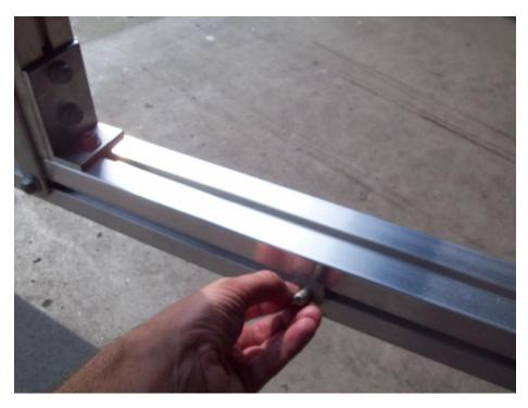
Install one repair T-bolt on each side of the tongue section toward the front on the trailer.
