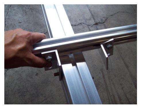
Attach mounting bar as shown, slide other angle bracket over, install nuts and tighten. Final position will be determined by box size.
