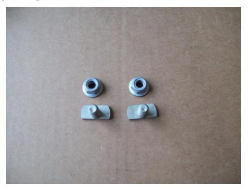
Locate two repair T-bolts and nuts.
