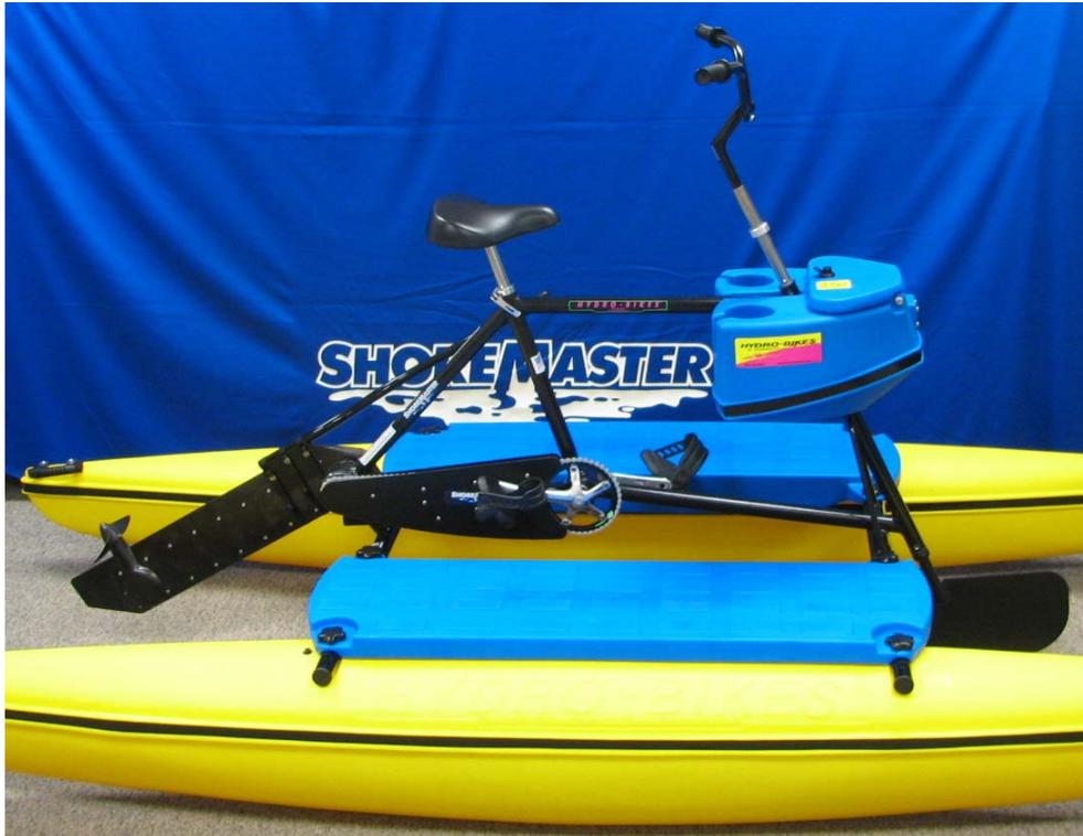
Attach console to Hydro-bike frame using two carriage bolts, four rubber washers and two large wing nuts. Use rubber washers on both sides of console.
